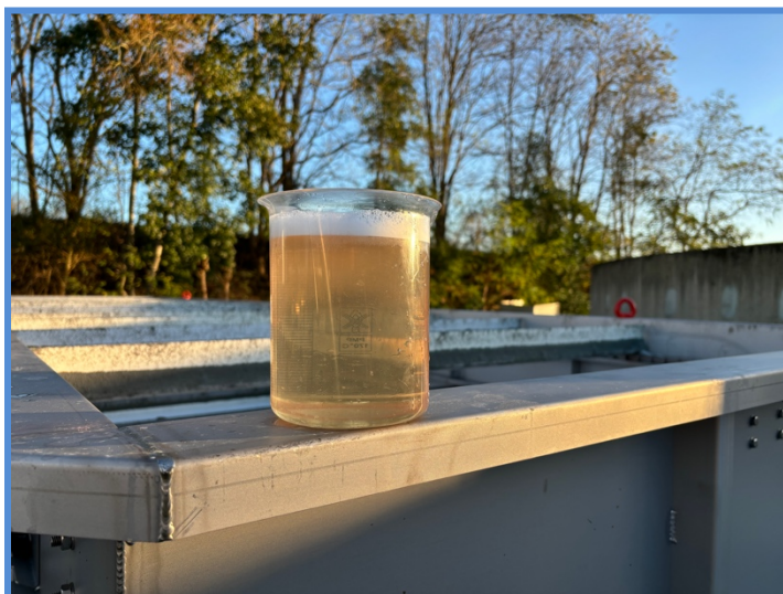
Photo 3: DAF effluent with less than 0,25 mg/l chrome
